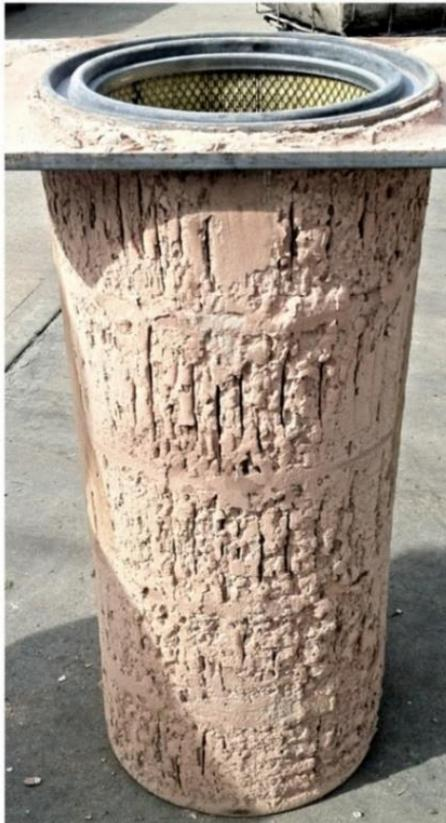
*Cartridge filter plugged up with dust*
