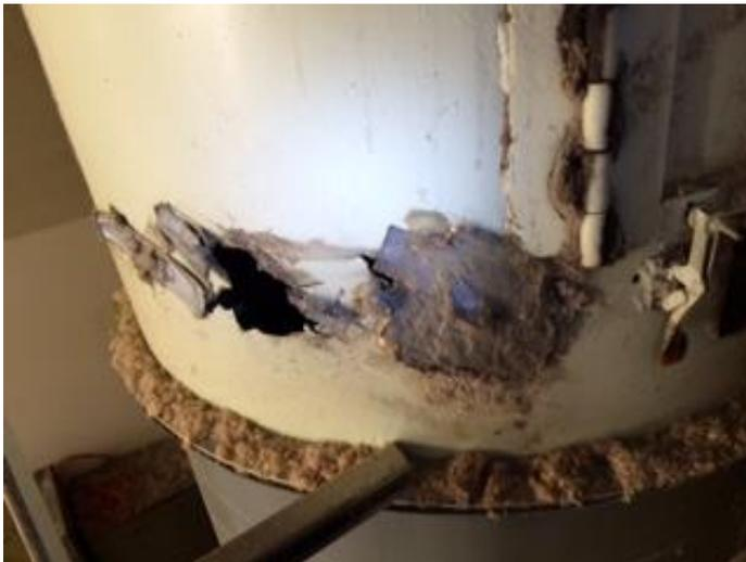
*Dust collector wear from corrosion / abrasion*
