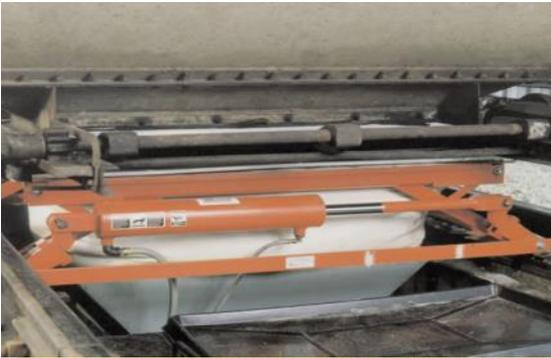
The **Boot-Lift® Railcar Connector** installs on the track flanges. Sponge seals fit securely to the hopper car unloading gates for a clean transfer of material to the under-track conveying system. No more material spillage on the tracks! Improves the safety of your employees, too. These connectors are fit to your needed dimensions.
